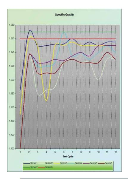
The real test of health in a battery is the specific gravity (SG) of the electrolyte. This was also measured over the same period of 24 days. The green line at 1.270 marks the 100% charged level, while the red line is the FAA minimum of 80%. The "Series 1 through 6" numbers are the cells being measured.
