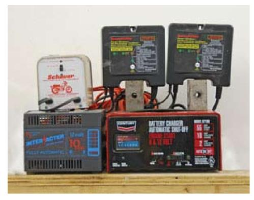
Five chargers and four levels of performance. Note also that the two chargers on the upper right are from BatteryMINDer. One is labeled is the 12248-AA-S3 for "Odyssey type" batteries, and the other is the S2, for conventional flooded-cell batteries. These chargers are designed for specific applications and, although they will work on, say, your car, for the best battery life the charger should match.
